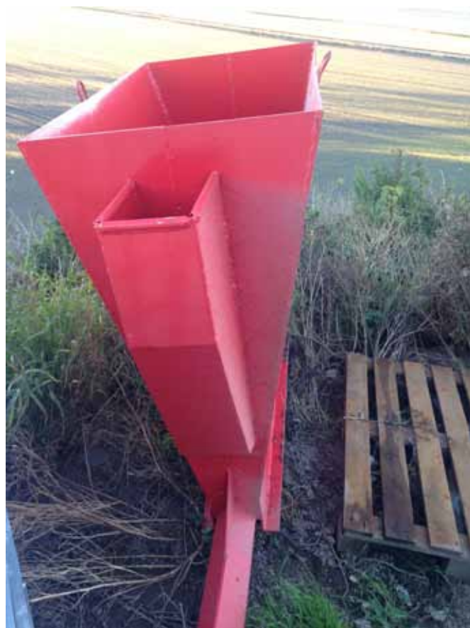
Grøftekasse for skuffegraving.
